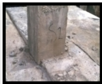
Tension side Compression side Figure (7): Crack pattern of slab S2
