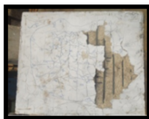
Tension side Compression side Figure (6): Crack pattern of slab S1
