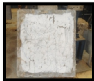
Tension side Compression side Figure (7): Crack pattern of slab S2
